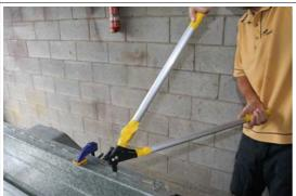
Fix the hinge to the trailer with heavy duty rivets.
