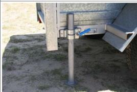
Use additional stabiliser legs to avoid tilting of the trailer.
