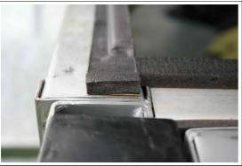
The sealing foam is placed on all 3 side walls and seals the gaps between the tent frame and trailer walls.
