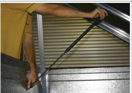
Once the mounting hinges are secured safely, click the gas struts back in (pistons facing upwards).
