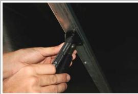
Put the mounting hinges onto the gas struts and mark the position you want to fix them on the tent frame.
