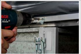
Fix the locking latches with self-drilling screws to the trailer walls and the steel frame of the tent.
