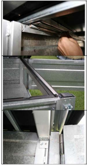
We recommend to fix the piano hinge directly onto the original tent frame.
