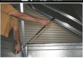
The gas struts need to be fixed to the metal frame of the tent and the side wall of your trailer.
