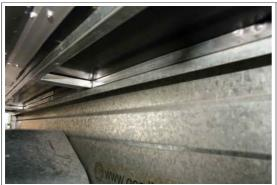
The remaining 3 tent steel frame sections should sit directly on your trailers side walls.
