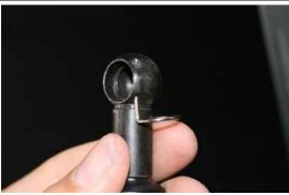
Open and remove the safety pin to attach or take off the strut.
