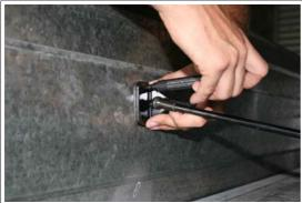
Mark the position of the gas strut hinges on the trailer side wall.
