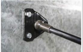
Use 6mm bolts, washers and split rings to fix the gas strut to the trailer wall.
