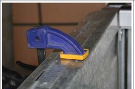
Place the hinge flat (NOT FOLDED) onto the trailer and fix it with clamps.
