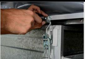
The two latches need to be placed on both corners opposite of the piano hinge.
