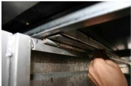
Align the tent frame with your trailer walls. The tent frame segment that connects to the piano hinge is made to sit slightly outside the trailer wall to connect to the flat piano hinge.
