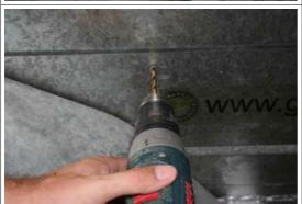
Drill 6mm holes to fix the gas strut hinges to the side wall of your trailer.
