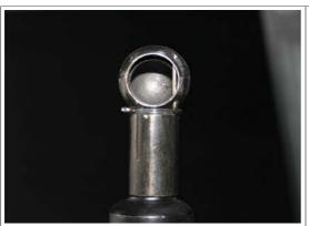
The gas struts have a safety pin on each side that locks the hinge to the head of the strut and prevents it from breaking free under force. It needs to be removed to attach or take the mounting hinges off.
